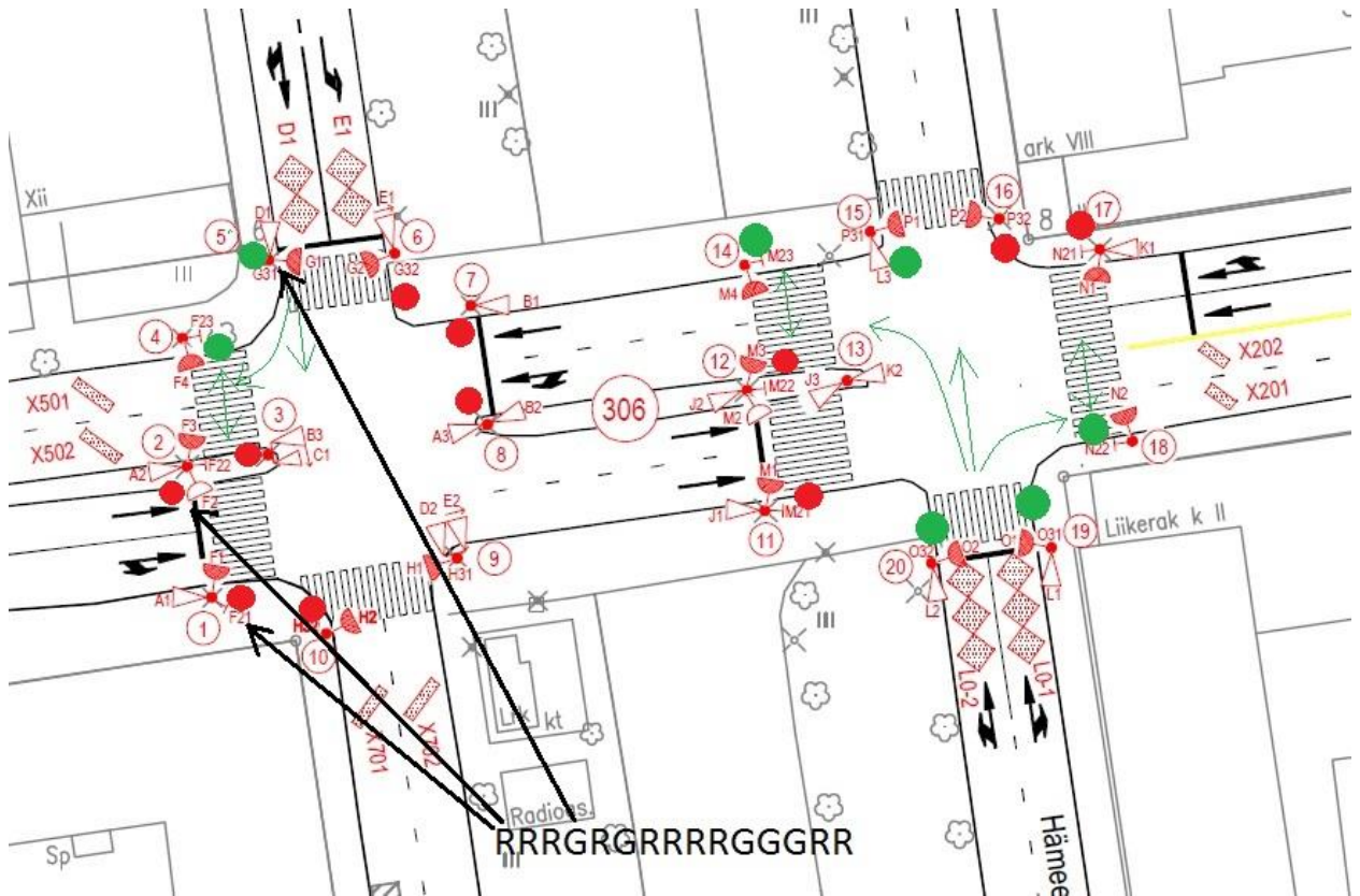
Figure 3. Signal states in the junction TRE306 at the timestamp 1445500407600.
